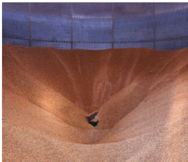
Earlier the two silos were sealed storage. Today they work as aeration silos with a filling rate of 3-4 times per year with storable grain.
